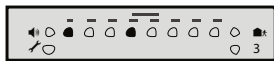
Active zones are indicated by the relevant zone lights on LED Keypads
